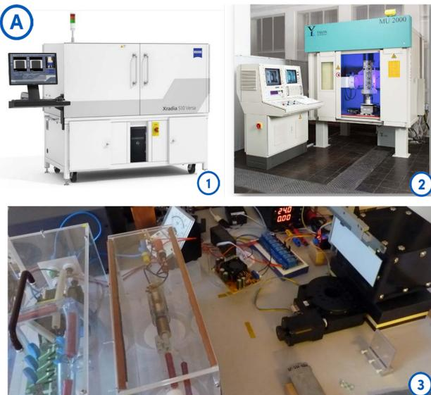
(1) HighQ Zeiss Xradia 510 [1μm res., 10W, 5s/img, high SNR]
